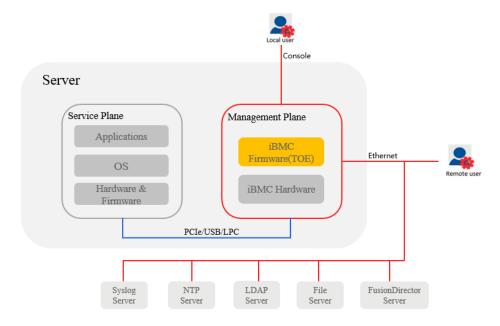
Figure 1-1 Operational environment of the TOE
